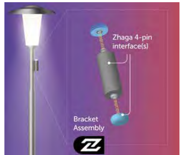
Figure 2: Zhaga Book 18 Ed 4 bracket assembly with interfaces for decorative and heritage luminaires.
